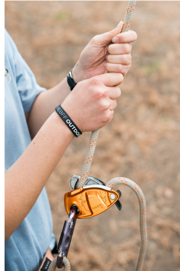
Make sure to perform pull test the GriGri + to ensure proper loading.
