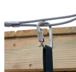
✗ Dead End of Cable with Serving Sleeve
