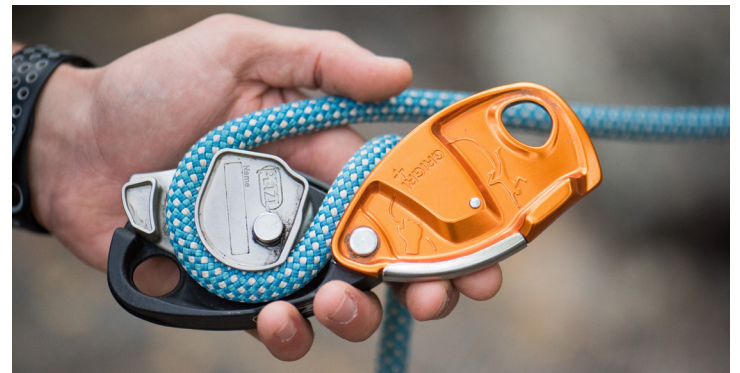
Proper loading of a GriGri +
