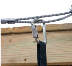
✗ Dead End of Cable with Serving Sleeve
