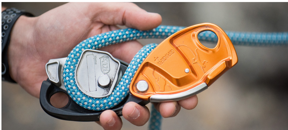
Proper loading of a GriGri +
