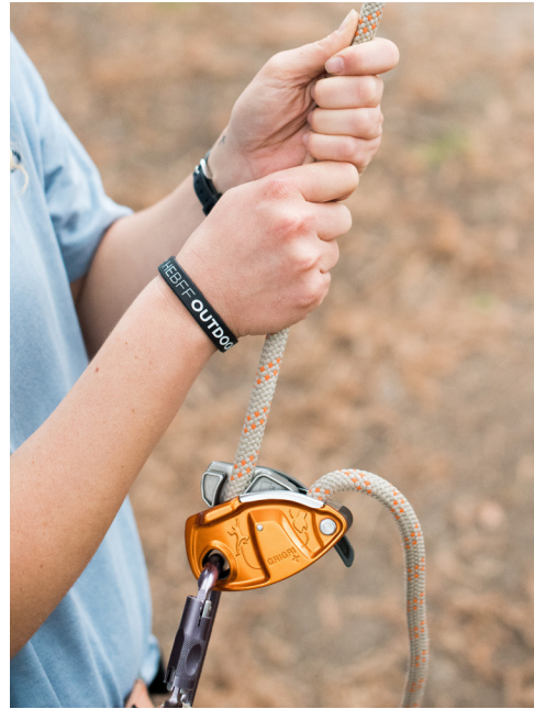
Make sure to perform pull test the GriGri + to ensure proper loading.
