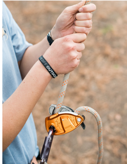
Make sure to perform pull test the GriGri + to ensure proper loading.
